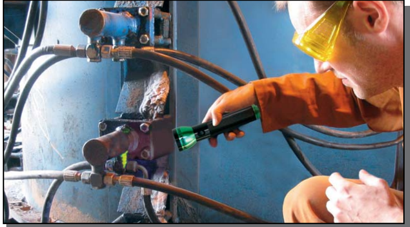
Leak checking valves and fittings with the OPTIMAX™ 3000 blue light LED flashlight
